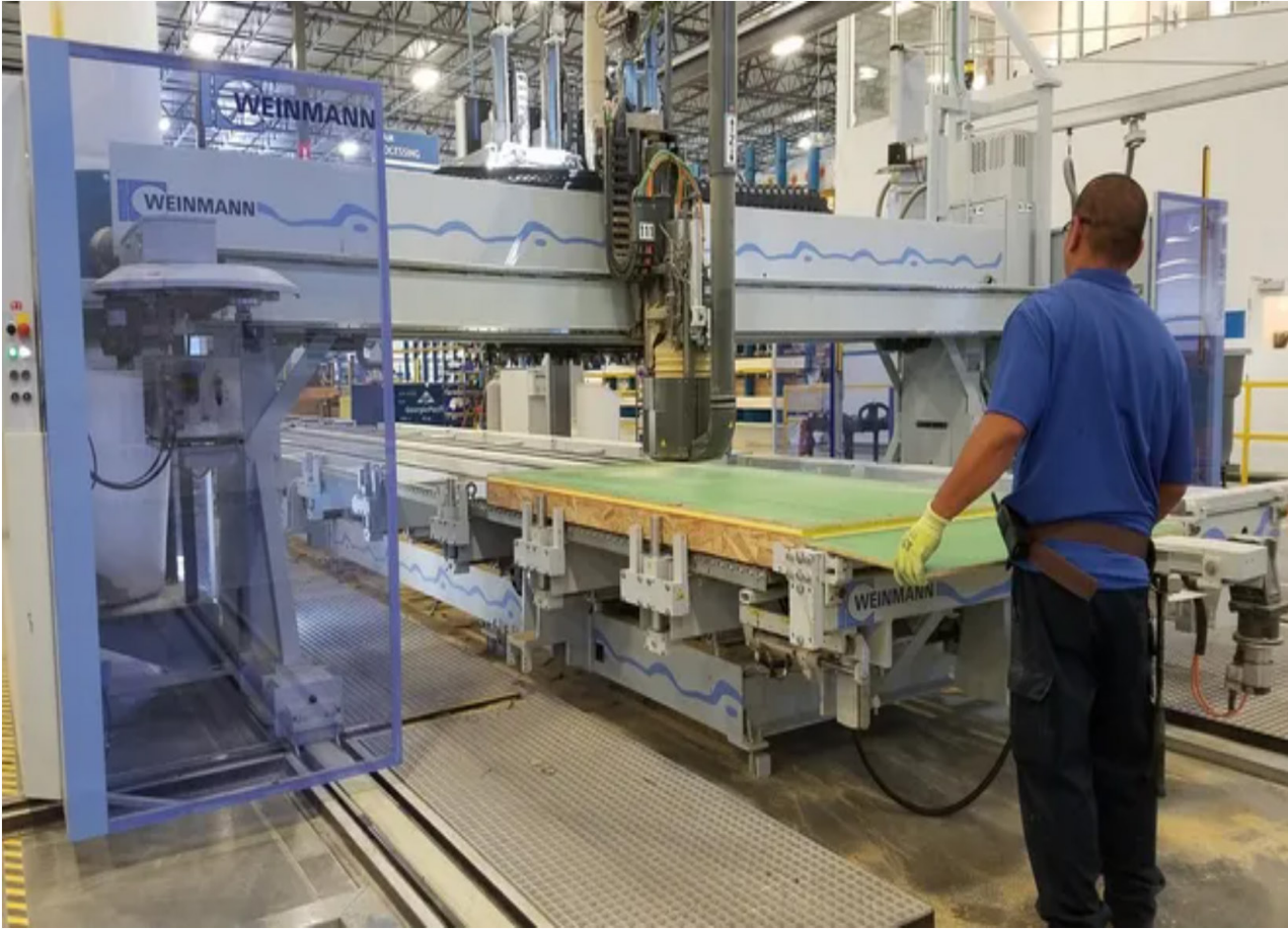
Photo shows Florante Fernando operating a wall processing machine which fastens, trims, and cuts openings in sheathing. Nick Panetta, Blueprint Robotics
