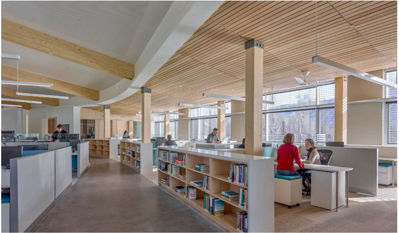
Open plan lets light penetrate and air circulate. Airflow is automated at the Innovation Center, meaning that nighttime flushes of stale air make the morning air fresh. Windows and exterior shading are automated for daytime cooling, heat gain, and ventilation. Photo taken at C on floor plan.
