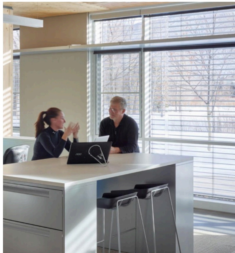
Exterior shading lets indirect light into the space while blocking unwanted direct sun, which can cause reflection and glare on screens. Photo taken at E on floor plan.
