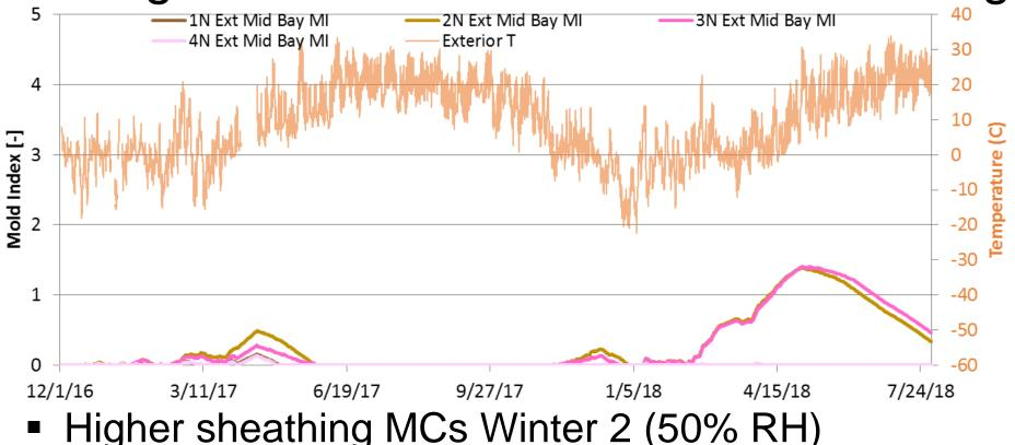
• Roof 4 RH sensor was drier than  $1/2/3 \rightarrow IOW MI$
