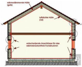
无热桥设计 Non-thermal bridge design
