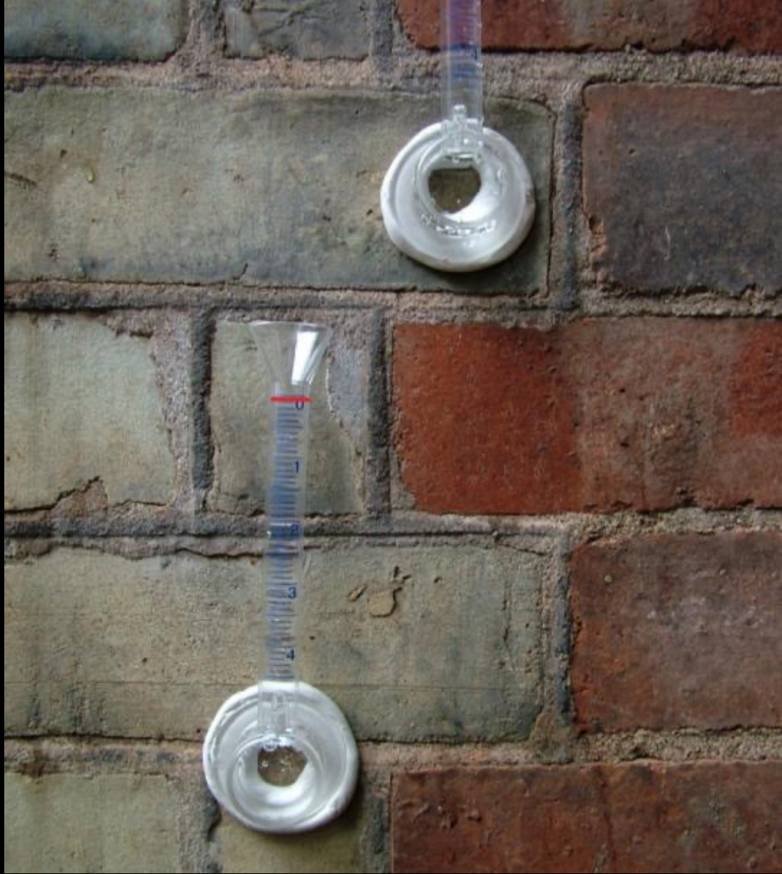
RILEM (AKA Karsten) tube moisture absorption test
