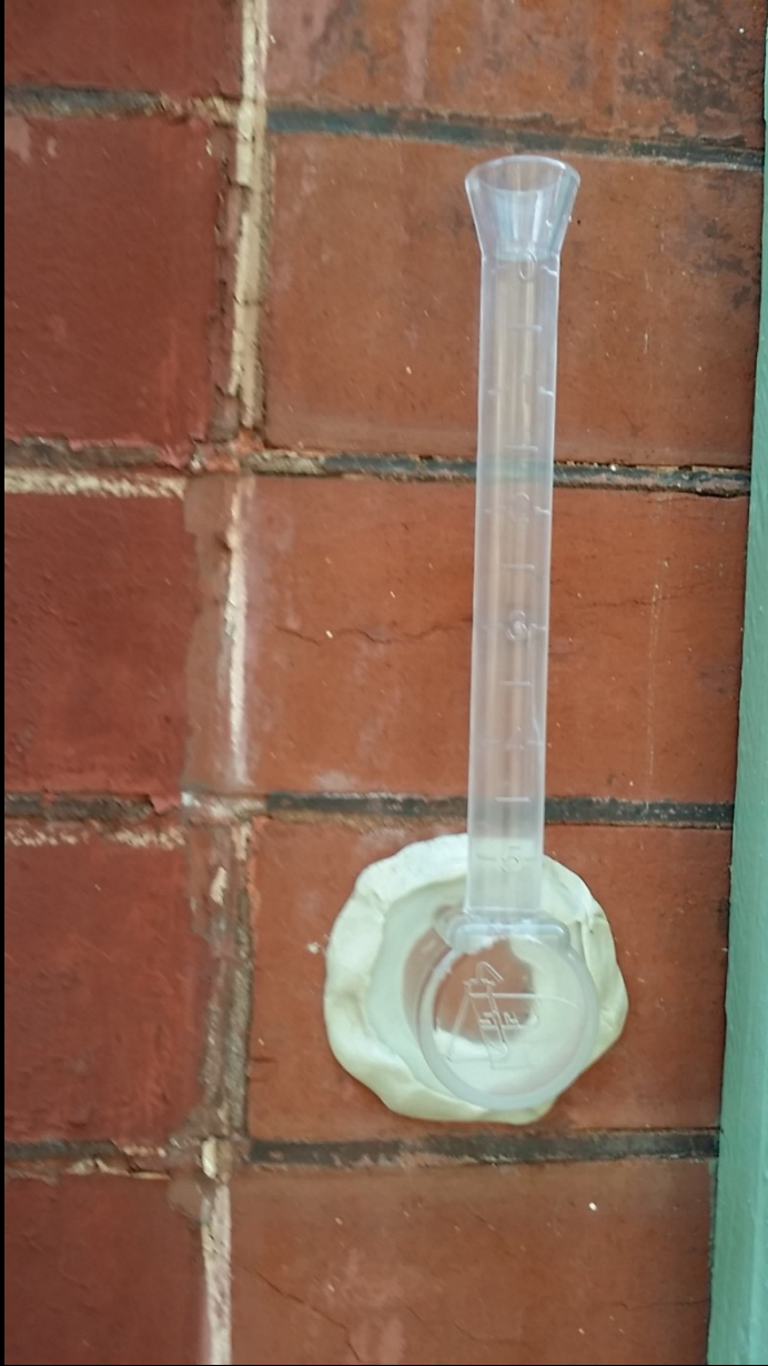
RILEM (AKA Karsten) tube moisture absorption test
