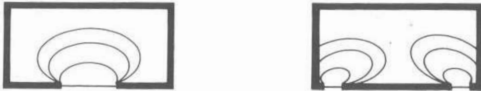
Figure 13.10b These plans, with contours of equal illumination, illustrate how light distribution is improved by admitting daylight from more than one point.
