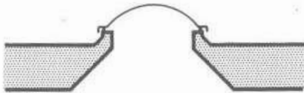
Figure 13.14c Splayed openings distribute light better and cause less glare than square openings.
