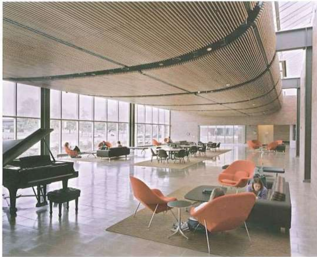
4.72 Multiuse room with toplighting and sidelighting to provide even daylight distribution at the Christopher Center at Valparaiso University, Indiana. © PETER AARON/ESTO
