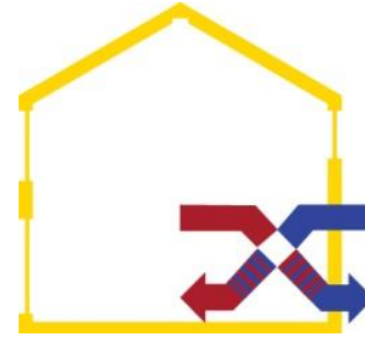
BALANCED VENTILATION WITH HEAT RECOVERY
