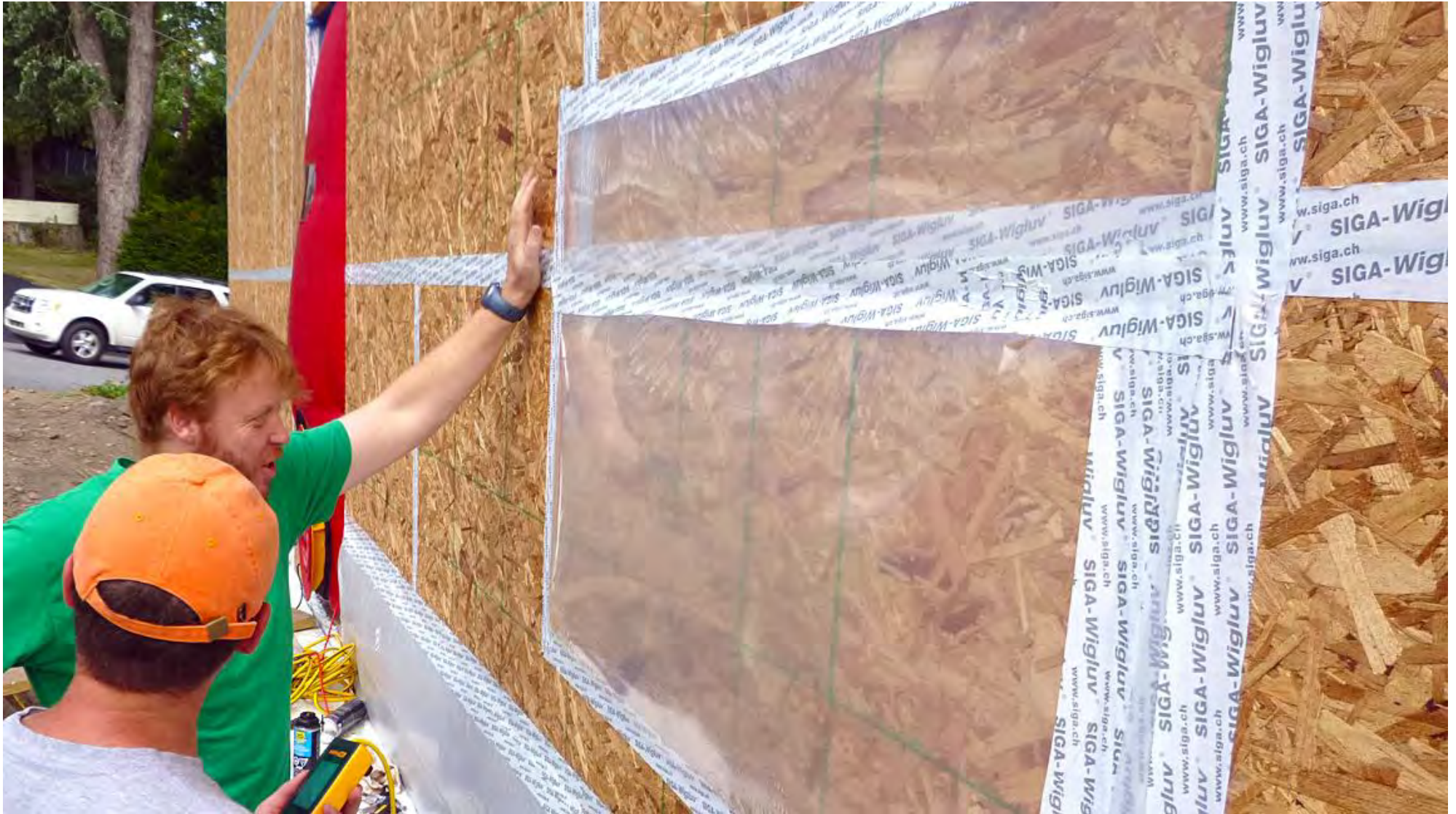
Balloon test #2 over OSB panel only
