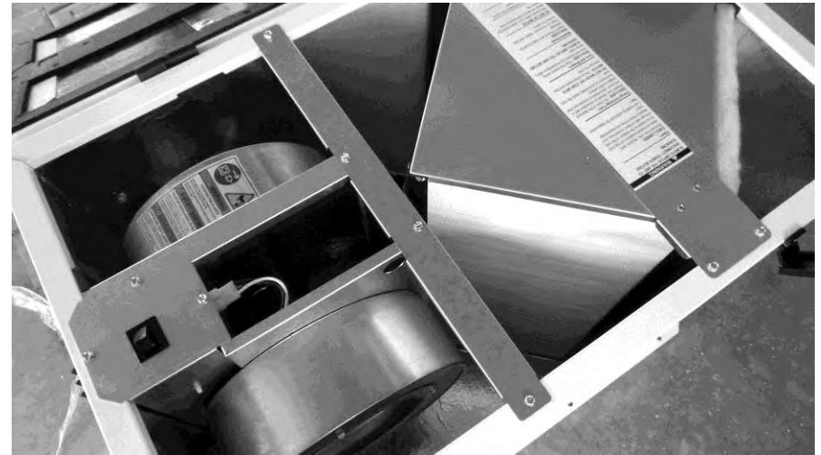
ERV single speed fan and Mitsubishi heat exchange core
