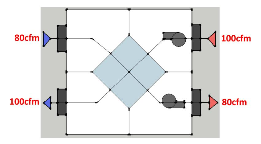
Intentional mass airflow imbalance during lab testing
