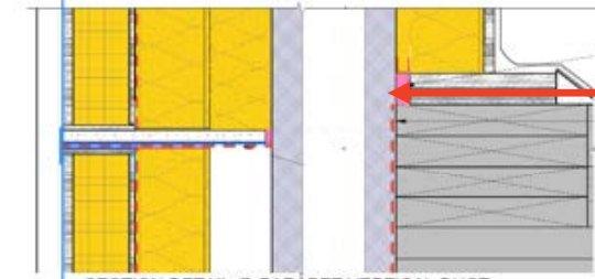
SECTION DETAIL @ PARAPET VERTICAL DUCT PENETRATION 13 3" = 1'-0"
